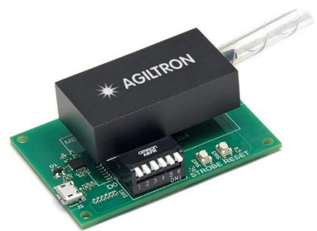
■ Mounted on USB/RS232/TTL PCB with Power Supply
